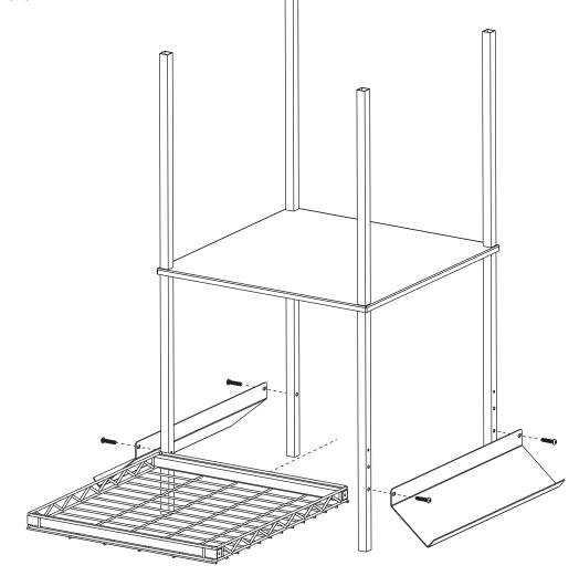
Note: The Wire shelf can be used as either a basket (as seen above) or flipped upside down for use as a flat surface.
