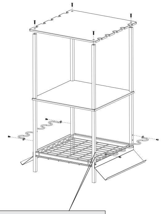
Note: The height of the Rod Holder (C) can be moved to either threaded hole depending on the desired height.
