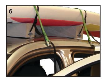
Unroll the two green 15' Load Straps. Open the vehicle's doors. Throw the non-buckle ends of each Strap up and over the SUP(s) and down to the other side of the vehicle.
