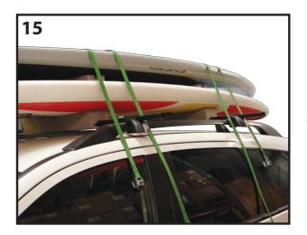
Both Load Strap loops should now be positioned over the SUP(s). See Image 15.
