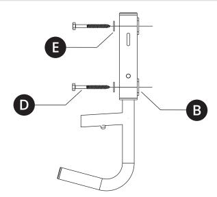
Install Arms (A) onto Frames (B) and secure via detent.
