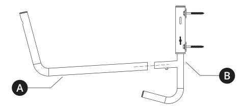
**Storage:** With the Arms (A) completely unweighted, pull the Quickpin (C), and swivel the arms 90 degrees to either side.
