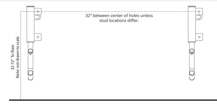
Using a 3/16" drill bit, drill 4 holes at the marked locations.
