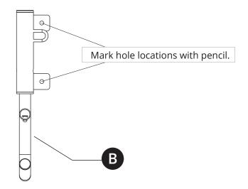
Measure from the floor to the center of the top hole pencil mark and note the measurement. Place the second Frame (B) 32" away and the same distance from the floor to the top hole as the other frame. Use a level to ensure holes line up vertically and mark the holes.
