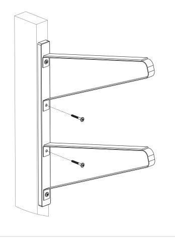
Note: If you want to have even spacing between the top and bottom section, you should have a gap of 1.5" between the two as seen to the right. This isn't required however, and if you would like to store an item that is taller, you should have a gap that allows these items to fit.
