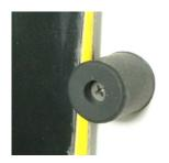
Step 3: Install the Rubber Bumpers: Place the wood screw in the rubber bumper such that the head of the screw will sink into the counter bore of the rubber bumper. Use a #2 Phillips driver, screw the bumper into the drywall anchor or other mounting surface. Remember to mount into X-mark.
