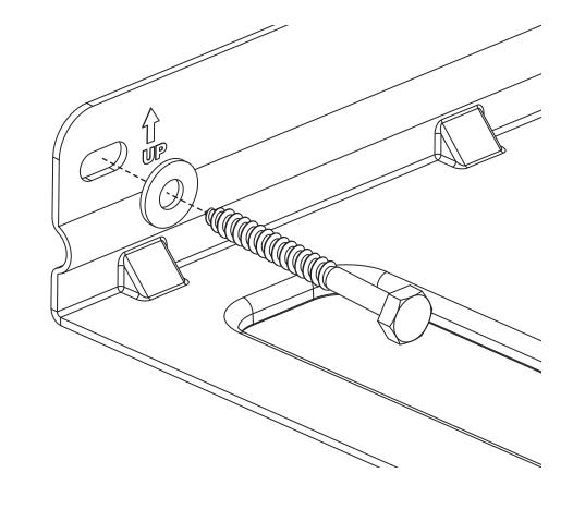
Repeat steps 1-4 to mount the Wall Shelf (B). Be sure to leave enough spacing between the Wall Shelf (B) and the Wall Rack (A) so are able to comfortably place items onto the Wall Rack (A) with no interference.
