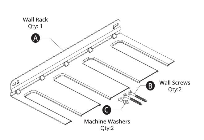
Use a stud finder to find two adjacent studs where you want to mount the product and mark the locations with a pencil. Hold the rack up to the wall where you want to mount it and align the mounting slots with the stud locations. Use a level to ensure the rack sits flat to the ground and mark both mounting slots along the studs.
