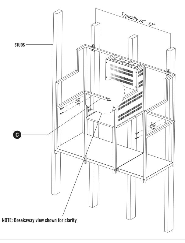
Secure the Strap Brackets (R) to the front of the rack using a bolt (K) and nut (Q). Tighten using the included allen key and a 8mm wrench.
