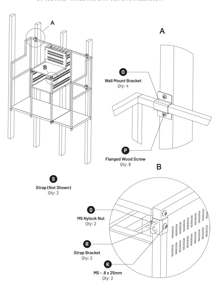
Use a stud finder to find two studs either 24" or 32" apart depending on the stud spacing of your wall. Mark the center of the two studs with a pencil at the height that you want the top of the rack to be. You may need to hold the rack up against the wall and have a friend make the mark.
