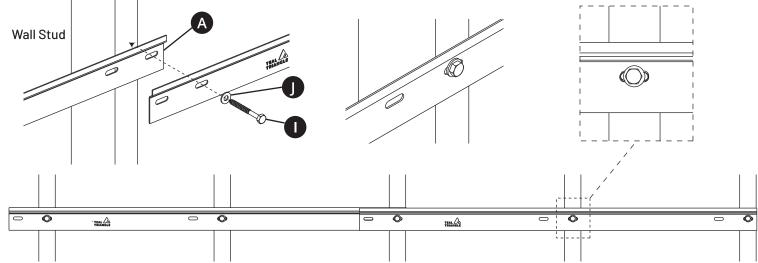
Hang the Vertical Tracks (B) from the Horizontal Rails (A) and line them up over the lag screws attached in the studs
