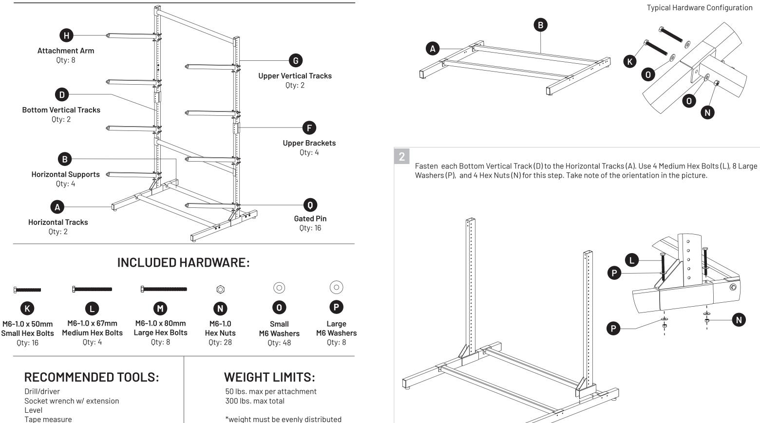
Assemble the third Horizontal Support (B) to both of the Bottom Vertical Tracks (D) at about the halfway point as seen below. Use 4 Small Hex Bolts (K), 8 Small Washers (O), and 4 Hex Nuts (N) for this step.
