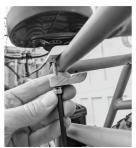
1. Determine which size clamp set you need for your application (measure with calipers or test fit with the parts)
