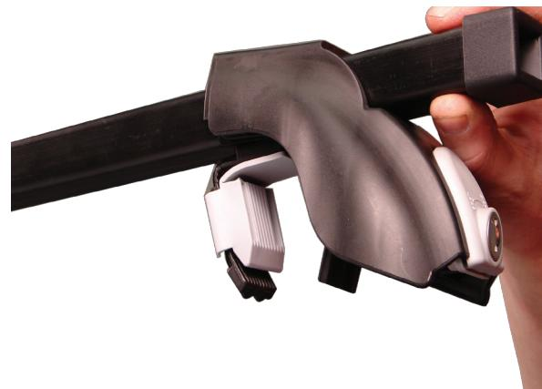
6). To complete the installation, insert the installation wrench and tighten the bolt clockwise until the feet hold the cross bars firmly in place. Apply pressure to confirm that no movement of the cross bars can be felt. Position the security shield into the tower and lock with key.
