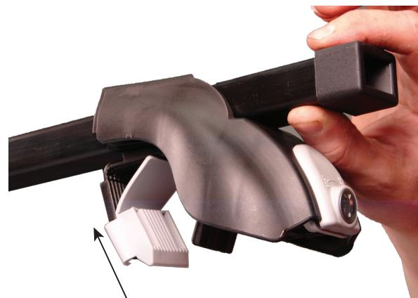
5). Push the rubber spacer block up each foot until the top flat section is formed around the top of the foot.
