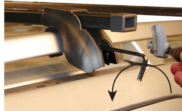
2). Lift the forward section of the tower to adjust it's position. Center towers over the raised side rails.
