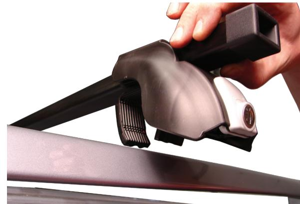
3). Place cross bars onto the vehicle's raised side rails. Adjust the distance between the bars for the load to be carried. Note: The bars must be separated by a minimum of 24".
