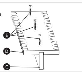
Assemble the components into one side as shown in the image. Align the components into the opposite side and assemble with the rest of the screws.
