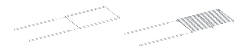
Align the crossbar (C) at the chosen height with the hole in the side (A). Using the included hardware, fasten the side (A) to the crossbar (C). Repeat for other shelf at desired height.
