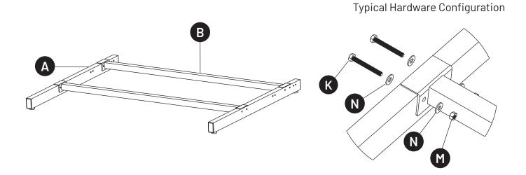
Fasten two Bottom Brackets (C) to each Bottom Vertical Track (D). Use 4 Small Hex Bolts (K), 8 Washers (N), and 4 Hex Nuts (M) for this step. Ensure the Bottom Brackets (C) are flush (side to side) with Bottom Vertical Tracks (D). Take note of the orientation in the picture. Note: The Bottom Vertical Tracks (D) do not have any end caps
