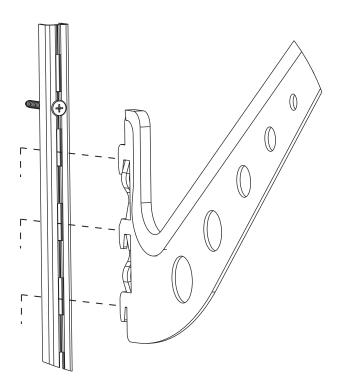
Once you are happy with the spacing of the Arms (A), and you confirm the line up between both Tracks, use a hammer or rubber mallet and gently tap down on the top of the base of each Arm to properly seat the Arms into each slot and reduce "wiggle".
